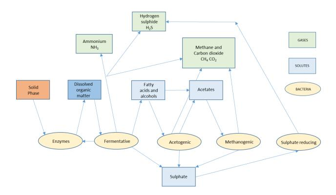
The processes involved in waste degradation are very complex and the literature on the subject contains a large number of versions of a block flow diagram of waste decomposition that attempt to describe what is happening. The diagram above is a simple version derived from one published by (Christensen and Kjeldsen 1989).
